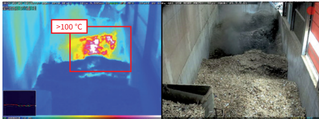
Thermal Radiometry (TR) automatically generates an alarm if the temperature exceeds or falls below the pre-defined temperature range.
